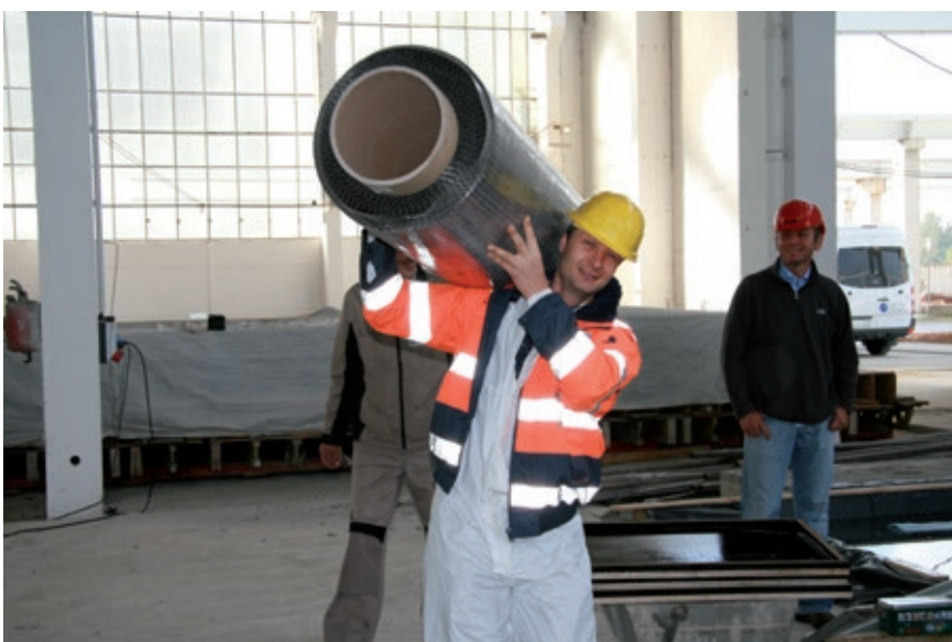
Fig. 3.3: “Light-weight” textile reinforcement, 25 m length / 1.25 m width
