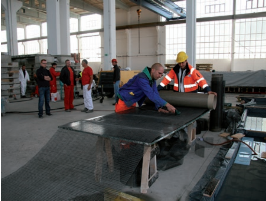
Fig. 3.5: Incorporation of textile in the fine concrete layer
